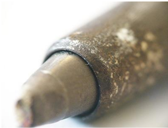
Close up view above of the nitrogen feed through the soldering iron collar to the tip of the iron on an alternative suppliers product
