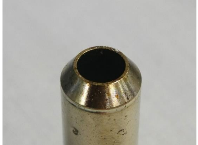
Close up around the soldering iron tip where nitrogen flows towards the soldering area during initial heating and soldering operation
