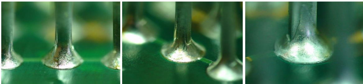
Three optical images above taken from gold over nickel boards soldered with SN96 solder wire using a system from mta Automation SA
