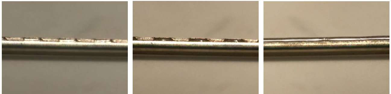
Three lengths of cored solder wire are shown, after placing on a hot plate set below the solder alloys reflow temperature. The three images show the flux rising in the indents created during wire feed and then flowing around the wire.
