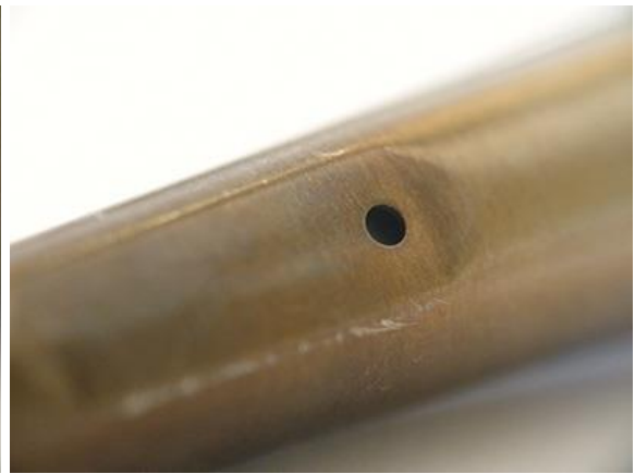
Close up view above of the nitrogen feed through the soldering iron collar to the tip of the iron on an alternative suppliers product
