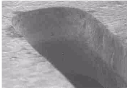
SEM section of Stainless steel etched stencil
