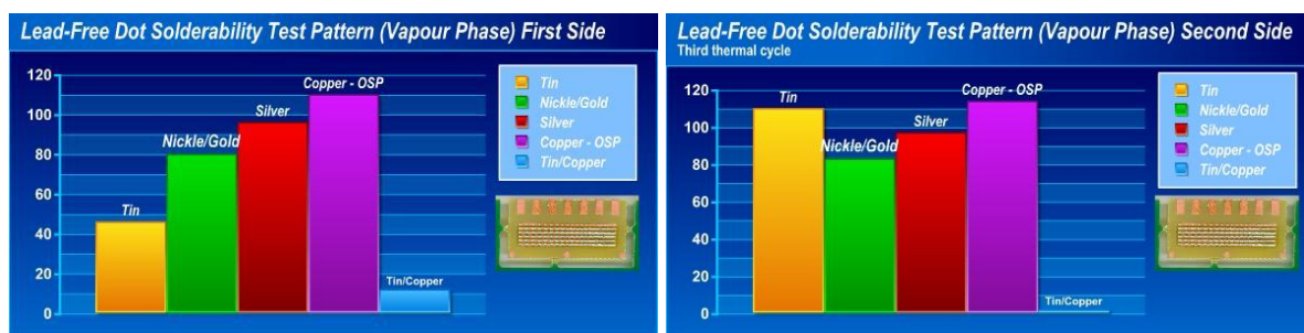
The graphs above show the change in wetting score after one and two reflows. Low scores on the graph are good and based on the solder paste wetting
