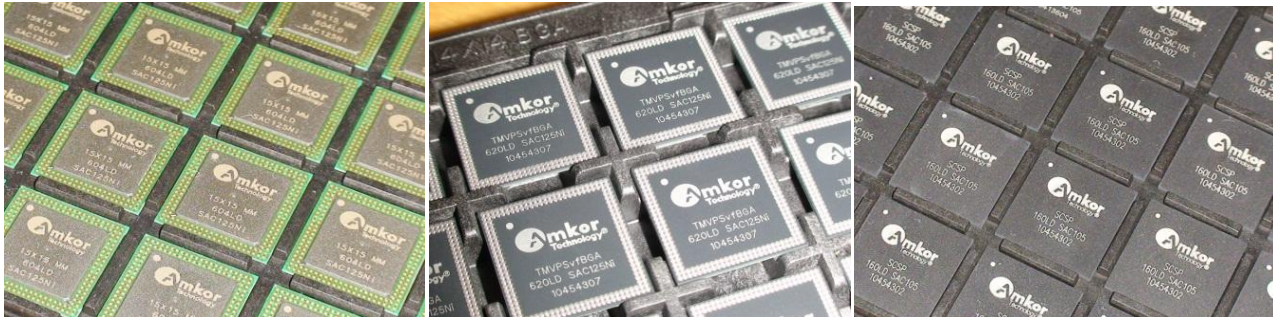
Selection of PoP parts in waffle trays provided for automatic assembly and used by the author during production trials and training sessions. In high volume the parts would be supplied in tape and reel format
