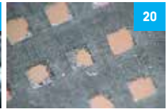
Poor Stencil Aperture Cleaning
