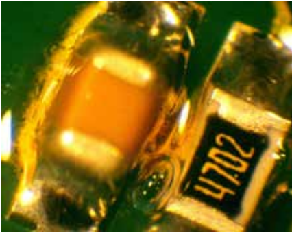
Coating lifting due to the chemical reaction on the board surface
