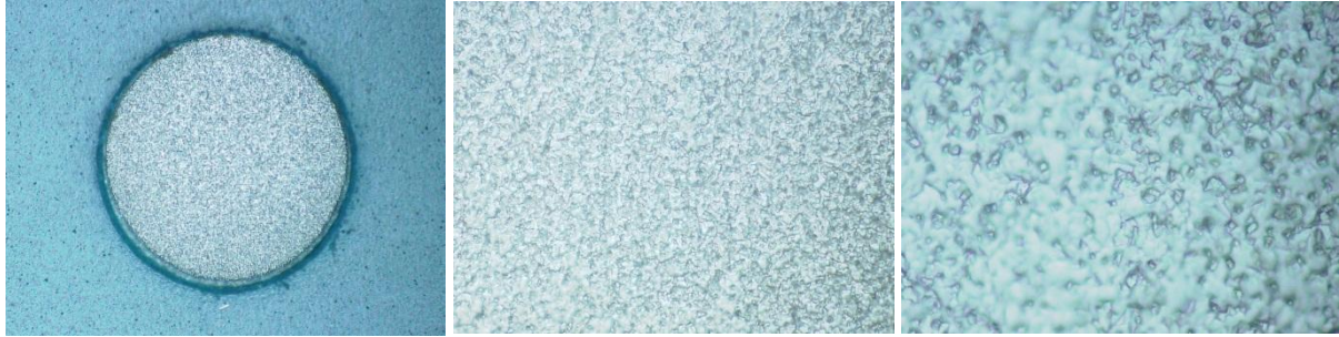
The images above show tin pads at 100, 500 & 100x magnification
