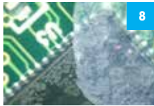
Mask De-wetting or Poor Adhesion
