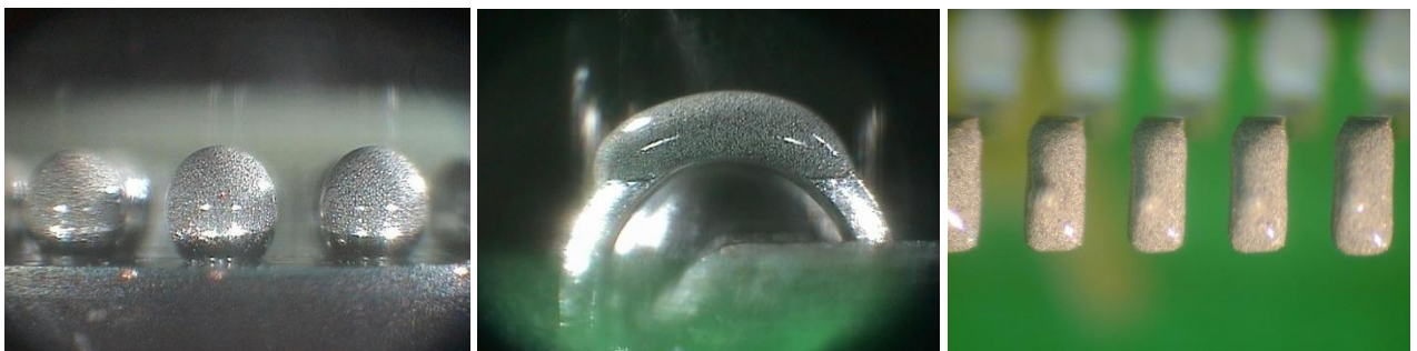
Dip solder paste can also be used for rework of standard BGA and other surface mount leaded devices as shown above. The parts have been dipped into paste and could then be placed and reflowed. Images show BGA (left), PLCC J lead (centre) and QFP gull wing (right)
