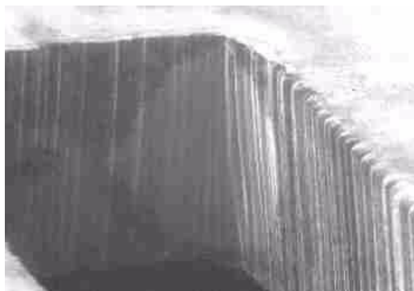
SEM section of electroformed stencil aperture
