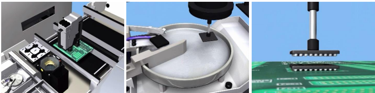
Video screen shots show images taken from a FUJI process animation. Images show placement of processor (left), dipping of memory device into paste (centre) and placement of memory device onto the processor (right)
