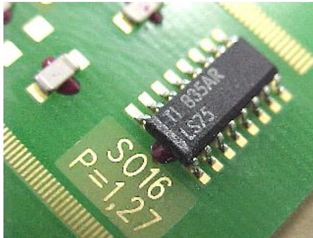
Practical examples of adhesive deposits being used on components during testing
