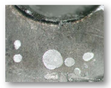
Surface of the pad on the joint failure above showing virtually no wetting or intermetallic bond. The solder around a plated through hole also shows evidence of separation from the base copper and is related to the PCB manufacturing process rather than any soldering operation
