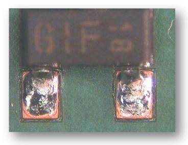
The choice of surface finish on a printed board will have an impact on degree of solder spread in tin/lead and leadfree assembly. The solder in the example has not wet over the full surface of the copper OSP pad but has formed a satisfactory joint. Exposed copper in many applications will not impact reliability; however, the difference in appearance, if not expected, can be an emotive subject with some customers
