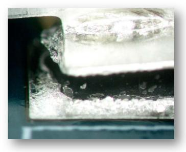
Solder joint failure due to the surface finish, the bulk of the solder on the component termination has separated from the pad after assembly. As the image shows, during reflow the solder paste has reflowed fully across the surface of the pads forming what visually would be a perfect joint. However the solder has failed to make a reliable connection. Investigation showed wetting to selected areas of the pads without fully wetting and forming an intermetallic layer across the joint
