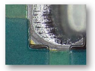
Solder paste has reflowed on the surface of the pad, consuming the gold and wetting to the nickel surface. The reduced wetting and coverage of the pad is related to the limited volume of the solder paste on the pad
