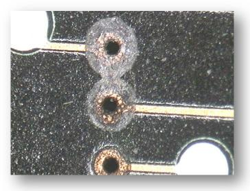
Corrosion deposits are visible around via holes on a product returned from the field. This could be related to creep corrosion due to the impact of sulphur and the product's working environment or trapped chemicals in the via holes not removed during manufacture. Surface analysis should be able to determine the failure type and is quite a common problem seen in industry, even if it does not cause immediate failure of a product
