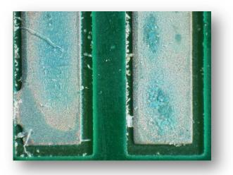
Solder mask residues are visible on the surface of the pads and may have been the result of a poorly controlled development and rinsing process, the imaging of the solder mask is well defined but with some undercutting of the solder mask. Ideally you will always have vertical side walls to avoid contamination and solder residues. Removing the residue showed the base pad surface
