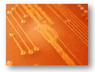
Solder levelling of flexible circuits normally requires a prebake of the circuit. Flexible circuits are made of polyimide and are far more prone to water absorption than normal epoxy/fibreglass substrates. Experience shows that baking can be avoided on single and double sided polyimide flexibles when a liquid solder mask is used as an alternative to a polyimide coverlayer
