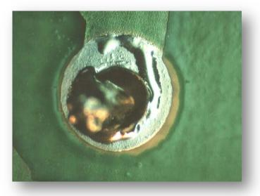
De-wetting of tin/lead solder on the surface of through hole pad may have been due to the copper pad preparation or the thickness of the solder coating in the original PCB manufacturing process. De-wetting is a less common defect today but is often misquoted in manufacture
