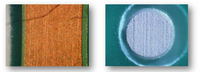
Any surface coating does not perform as well if the copper surface below is subjected to a mechanical cleaning operation. The score marks on the surface of the pad are plainly visible on this copper OSP board. The poor surface treatment of the copper surface has been shown to impact the storage life of organic coatings as well as tin and silver and should be investigated. The mechanical cleaning marks are less obvious on the pad of the silver finish sample shown on the right
