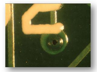
When solder mask is applied over a via hole sealing the barrel outgassing can cause the resist to pop during solder levelling. The resist blister may seem just a cosmetic problem but it can affect solder paste printing on fine pitch boards. The resist locally lifts the stencil from the surface of the board. The appearance of lifting or cracking of the solder mask may be affected by the type of mask, one that is either brittle or flexible
